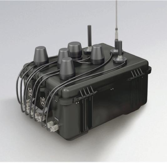
The jammer serves to interfere with the operation of the radio-controlled explosive devices (RCED) by means of a signal within the operating frequency band; the jammer is designed to provide protection against **RCED** when moving and in the stationary position. The device is used in a dense urban development when it is required to quickly change the safety zone location. The jammer is made as a case.
