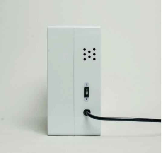
The jammer is designed to counteract cellular communication of GSM 900/1800, 3G, 4G-700, 4G/LTE and WiFi standards in individual limited areas.
